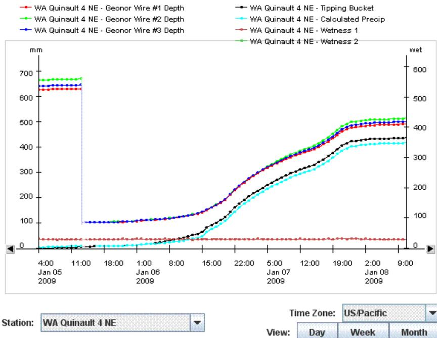
measure the large precipitation event. The depth rose to nearly 500 mm in just two days, and could have potentially over-topped the gauge if it were not drained before the event. This reflects the need for prompt responses to requests for gauge drainage or other less routine remedial actions that are important for the preservation of accurate and continuous observations for stations in the USCRN. We certainly appreciate the dedication of all our site technical contacts.
